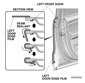
15. Using a shop towel, wipe the excess 3M protective tape application solution from the left door edge film. Allow the left door edge film to dry thoroughly.
