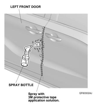
4. Using a spray bottle with the 3M protective tape application solution, spray the outside of the left front door where the left door edge film will attach. NOTE: Do not spray the inner surface.
