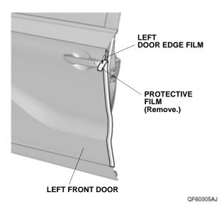
14. Starting from the center and working outward, use your fingers to fold the left door edge film around the edge of the left front door. Move your fingers in one direction. Attach the left door edge film over the seam sealant. Do not trim or damage the seam sealant.
