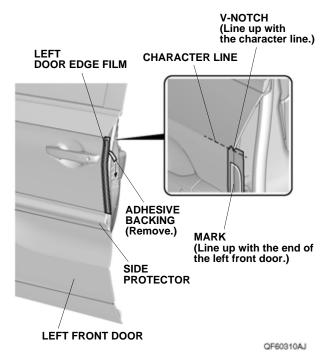
Line up the mark on the upper part of the left door edge film with the end of the left front door. While applying light pressure, carefully remove the adhesive backing. 10. Peel back about 50 mm (2.0 in.) of adhesive backing from the lower part of the left door edge film. Line up it with the side protector on the left front door.
