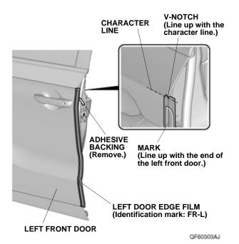
Line up the mark on the left door edge film with the end of the left front door. While applying light pressure, carefully remove the adhesive backing. Then, go to step 12.
