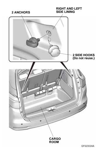
3. Install the cargo net onto the anchors and side hooks as shown.
