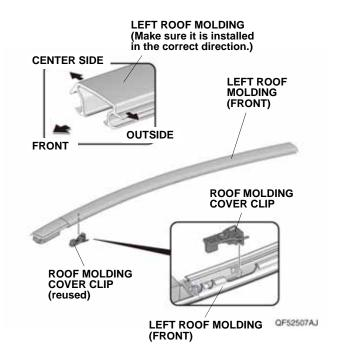
Install the molding clip to the left roof molding (rear).
