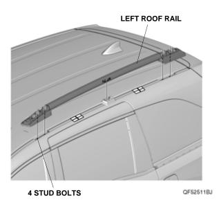
12. Install the four TORX nuts and two TORX bolts.
