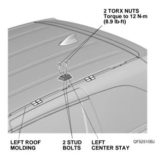
11. Place the left roof rail over the four remaining stud bolts.
