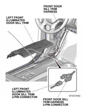
22. Using scissors, cut the urethane tape as shown. Wrap the urethane tapes around the 2-pin connectors.
