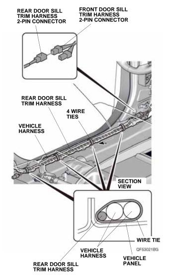
31. Route the rear door sill trim harness along the vehicle harness, and secure it to the vehicle harness with four wire ties.
