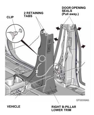
Pull away the door opening seal, and remove the driver's dashboard side lid.
