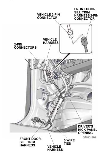
20. Route the front door sill trim harness along the vehicle harness, and secure it to the vehicle harness with two wire ties.
