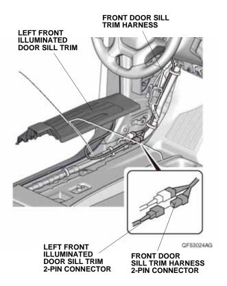
42. Using scissors, cut the urethane tape in half, and attach the two halves of urethane tape to the 2-pin connectors as shown.
