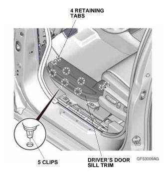
14. Pull away the door opening seal, and remove the driver's kick panel.
