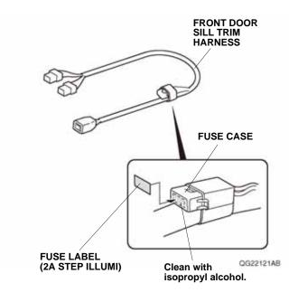
19. Plug the vehicle 2-pin connector into the front door sill trim harness 2-pin connector, and secure the 2pin connectors to the vehicle harness with one wire tie.
