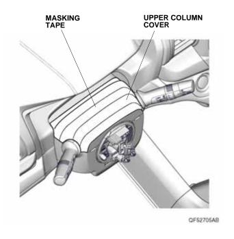
12. Using a plastic trim tool, release two retaining tabs.
