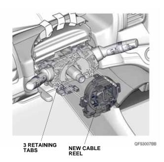
22. Plug the vehicle connectors into the new cable reel, and remove the locking pin.
