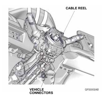
17. To prevent turning from the cable reel, apply masking tape to the cable reel. Remove the cable reel.
