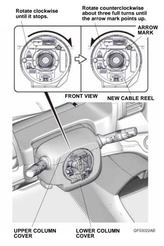
37. Before installing the new steering wheel, make sure the front wheels are pointing straight ahead, then center the new cable reel. Do this by first rotating the new cable reel clockwise until it stops, then rotate it counterclockwise about three full turns. The arrow mark on the new cable reel label should point straight up.
