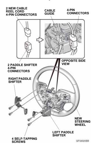
35. Install the steering wheel cover on the new steering wheel with the four self-tapping screws removed in step 23 and two retaining tabs.
