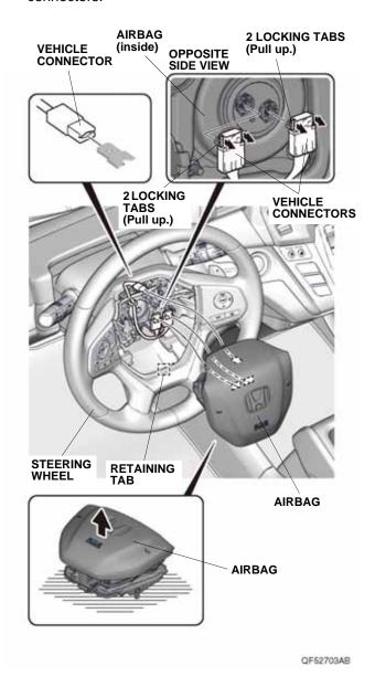
7. Remove the airbag. Do not drop the removed airbag or hit it on an object. Place the removed airbag in a safe place with the pad surface (top) facing upward.
