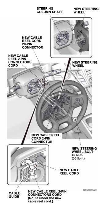
39. Install the new steering wheel bolt. Torque the new steering wheel bolt to 49 N·m (36 lb·ft). Tighten at the specified torque within 5 minutes.
