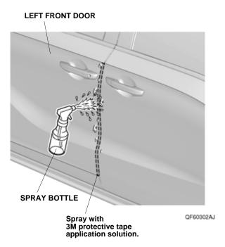
4. Using a spray bottle with the 3M protective tape application solution, spray the outside of the left front door where the left door edge film will attach.
