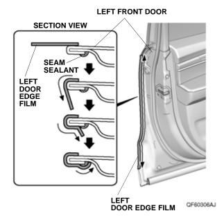
15. Using a shop towel, wipe the excess 3M protective tape application solution from the left door edge film. Allow the left door edge film to dry thoroughly.
