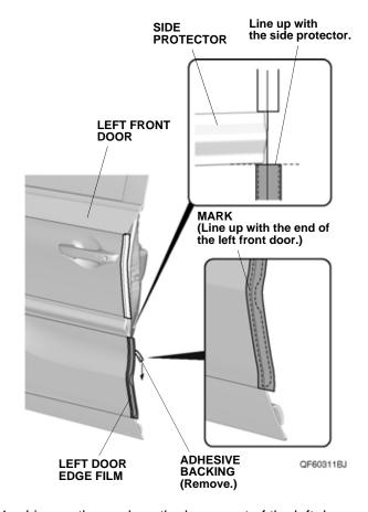
Line up the mark on the lower part of the left door edge film with the end of the left front door. While applying light pressure, carefully remove the adhesive backing.
