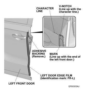
6. Line up the mark on the left door edge film with the end of the left front door. While applying light pressure, carefully remove the adhesive backing. Then, go to step 12.
