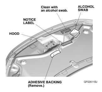
13. Remove the adhesive backing from the notice label, and attach it to the hood as shown.
