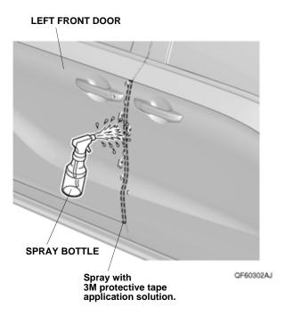
Using a spray bottle with the 3M protective tape application solution, spray the outside of the left front door where the left door edge film will attach. NOTE: Do not spray the inner surface. If the vehicle is equipped with side protectors, go to step 7; otherwise, continue with step 5.
