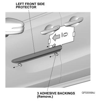
10. Using the rubber roller, apply firm pressure while rolling, especially at the ends, to set the adhesive.
