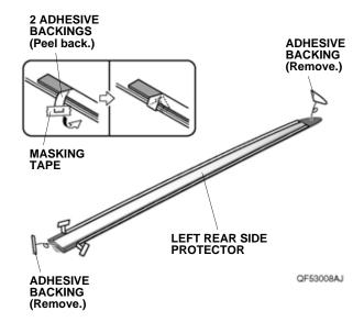
Line up the left rear side protector with template A and template B, and install the left rear side protector on the left sliding door.
