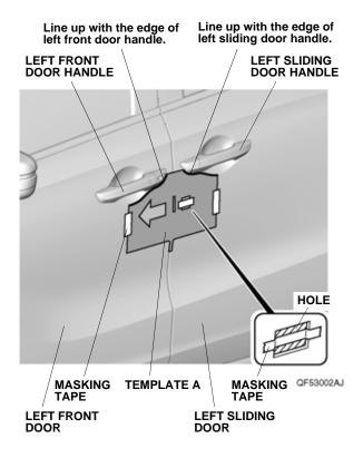
Line up template B with the edge of the left sliding door, making sure the arrow hole points to the rear of the vehicle. Then, attach template A to the left sliding door with masking tape as shown.
