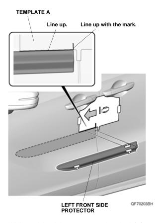
While applying light pressure against the left front side protector, carefully remove the taped adhesive backings.
