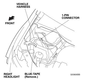
15. Plug the fog light harness 1-pin connector to the vehicle 1-pin connector.
