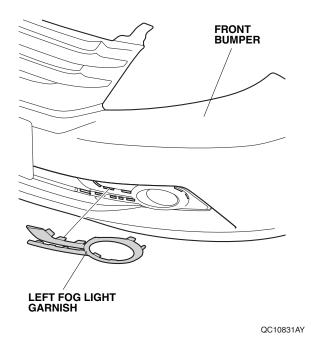
31. Secure the left fog light to the front bumper with one 5 x 16 mm washer-bolt.
