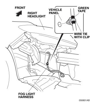
20. Secure the fog light harness to the vehicle harness with two wire ties.
