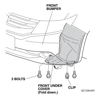
Insert your hand inside the under cover, and unplug the vehicle connector from the left fog light. Remove the bulb.
