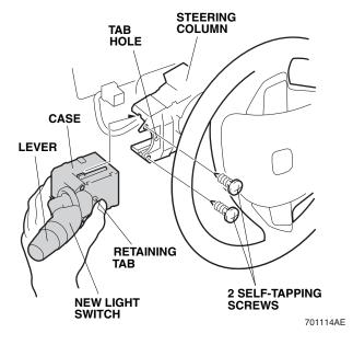
40. Plug the light switch connector into the new light switch. Make sure the vehicle harness is not being stretched.
