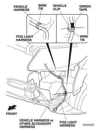
24. Secure the fog light harness to the vehicle harness with one wire tie. Go to step 27.
