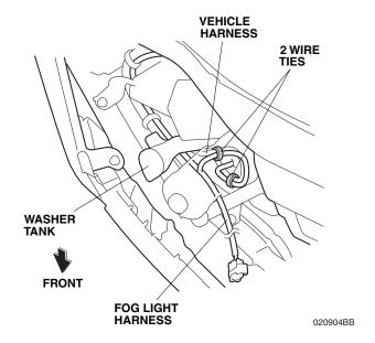
21. Route the fog light harness along the vehicle harness, and secure it to the vehicle harness with six wire ties.
