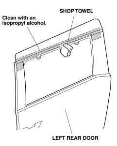
15. Peel back 1½ to 2 inches of each adhesive backing, and tape the ends to the front surface of the left rear door visor with masking tape.
