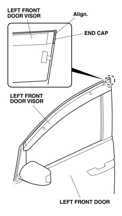
While applying light pressure against the left front door visor, carefully remove the adhesive backings.
