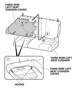
Secure the third row left seat cushion cover to the third row left seat cushion with the two hook-andloop fasteners.
