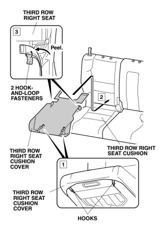
11. Secure the third row right seat cushion cover to the third row right seat cushion with the two hook-and-loop fasteners.
