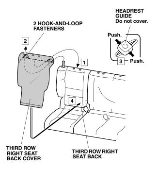
9. Fold down the third row right seat. Secure the third row right seat back cover to the third row right seat back with one hook-and-loop fastener. Return the third row right seat to the upright postion.
