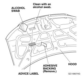
Remove the adhesive backing from the advice label, and attach the advice label to the hood as shown.
