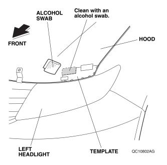
7. Remove the adhesive backing from the bracket C, and align it to the template secured in step 5. Remove the template.
