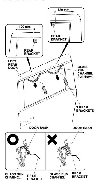
13. Reinstall the glass run channel to secure the two rear brackets. Be sure the brackets are installed tightly to the door sash, and that the glass run channel is properly seated.
