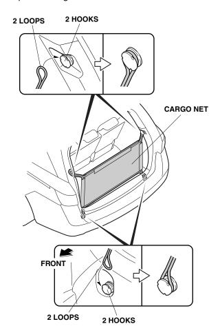
2. Secure four loops on the cargo net to the four hooks in the vehicle as shown.
