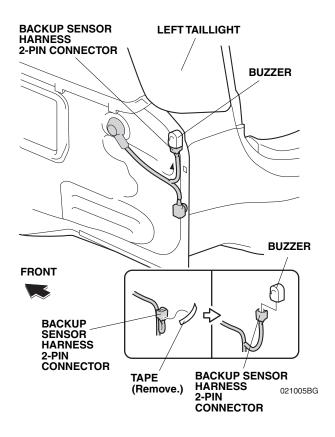
66. Route the vehicle 2-pin connector, and plug it to the backup sensor harness 2-pin connector.
