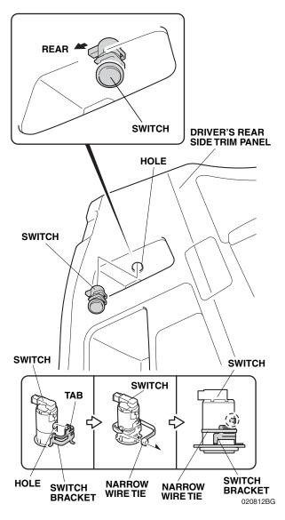
34. Align the tab on the switch bracket to the hole on the switch and secure the switch bracket to the switch with one narrow wire tie.
