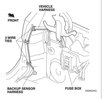
45. Route the backup sensor harness 2-pin connector along the vehicle harness.
