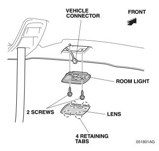
8. Remove the room light (two screws and unplug the vehicle connector).
