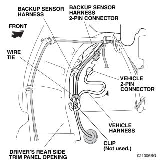
67. Secure the vehicle harness and backup sensor harness to the vehicle harness with one wire tie as shown.
