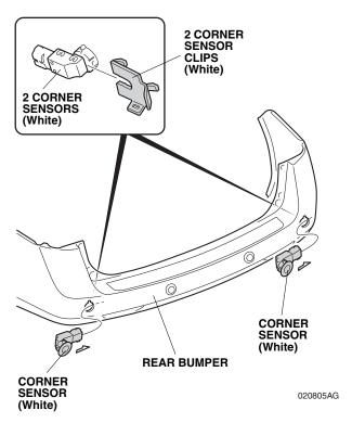
23. Secure two corner sensors (White) with two corner sensor clips (White) as shown.
