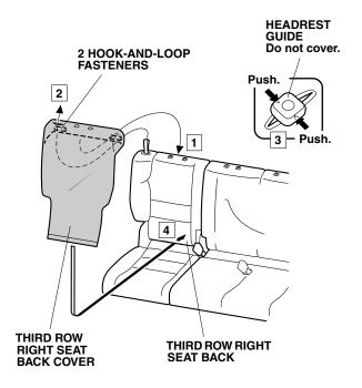
9. Fold down the third row right seat. Secure the third row right seat back cover to the third row right seat back with one hook-and-loop fastener. Return the third row right seat to the upright postion.
