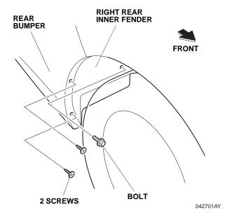
4. Secure the right rear splash guard to the right rear inner fender and rear bumper with one hook, one 5 x 25 mm self-tapping screw, one bolt removed step in 3 and one screw removed step in 3. While holding the splash guard firmly against the fenderwell, tighten the self-tapping screw, screw and bolt in the order 1→2→3.
