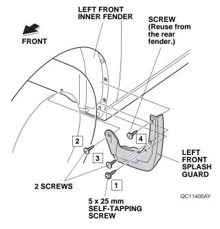
9. Turn the steering wheel fully clockwise, and repeat steps 6 through 8 to install the right front splash guard.
