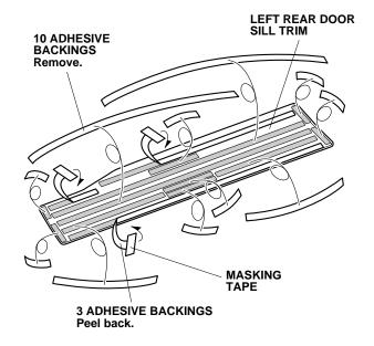
19. Remove the remaining adhesive backings.
