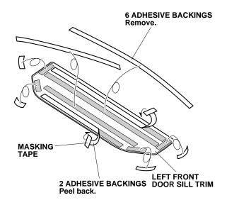
8. Remove the remaining adhesive backings.
