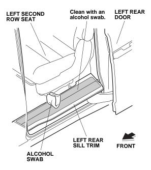
Attach masking tape to the left rear sill trim as shown.
