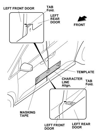
3. Align the bottom of the template with the character line, and attach the template to the left doors with strips of masking tape as shown.
