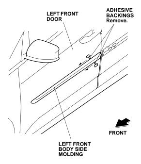
9. Using a rubber roller, apply pressure against the left front body side molding and roll from one end to the other.
