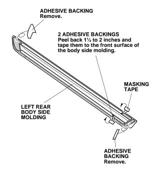
11. Align the left rear body side molding with the template and attach it to the left rear door as shown.
