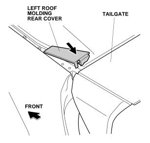
Reinstall the cut pieces of the left roof molding onto the roof of the vehicle as shown.
