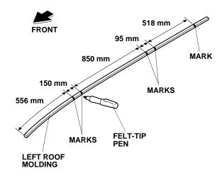
7. While wearing eye protection, use an air saw to cut off the left roof molding at the marks made in step 6.
