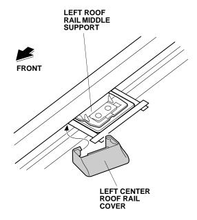
18. Install the left center roof rail cover to the left roof rail middle support as shown. Make sure there is no clearance between the left center roof rail cover and the left roof rail middle support.
