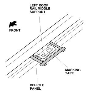
17. Hook the left center roof rail cover to the left roof rail middle support as shown.
