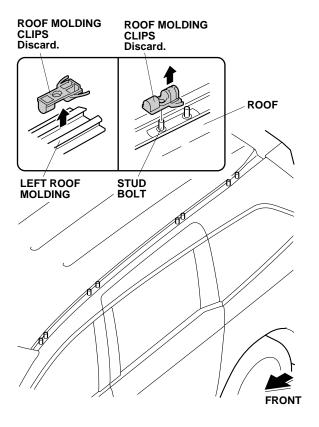
5. Remove any sealant that is on the base of the stud bolts.
