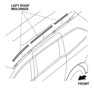
Install the left side roof rail with six Torx nuts. Make sure the roof rail is installed in the correct position. Torque the Torx nuts to: 10 N·m (7.3 lbf·ft)
