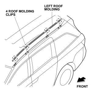
2. Open the tailgate halfway. Using a trim tool, pry up the rear of the left roof molding rear cover.
