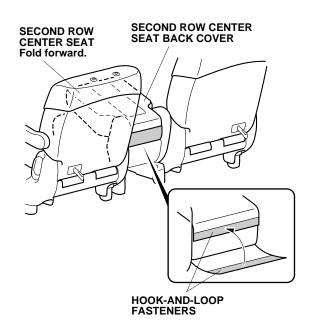
11. Secure two hook-and-loop fasteners on the second row center seat back cover as shown.
