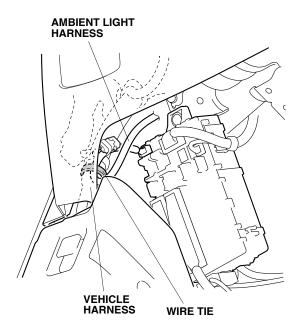
Install the ambient light into the hole in the dashboard as shown.
