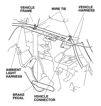
Route the ambient light harness through the center console, and secure it to the vehicle harness with three wire ties. Secure the wire tie next to the vehicle clip.
