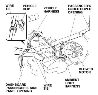
16. Secure the ambient light harness to the vehicle harness with three wire ties. Secure the wire tie next to the vehicle clip.
