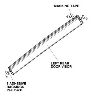
16. Place the door visor against the door, and adjust the visor so it lines up with the two rear brackets.
