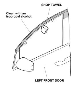
5. Peel back 1½ to 2 inches of each adhesive backing, and tape the ends to the front surface of the left front door visor with masking tape.
