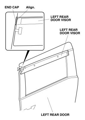
While applying light pressure against the left rear door visor, carefully remove the adhesive backings.
