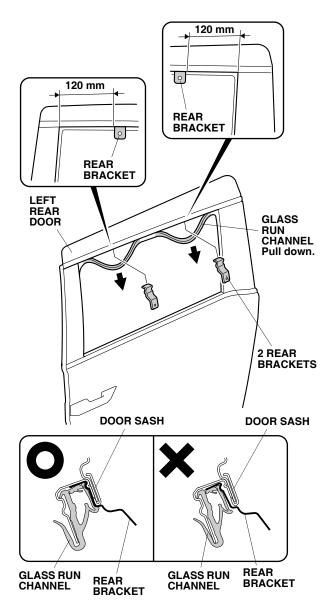
Reinstall the glass run channel to secure the two rear brackets. Be sure the brackets are installed tightly to the door sash, and that the glass run channel is properly seated.
