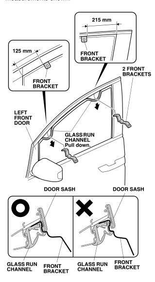
Reinstall the glass run channel to secure the two front brackets. Be sure the brackets are installed tightly to the door sash, and that the glass run channel is properly seated. 4. Using isopropyl alcohol on a shop towel, thoroughly clean the door where the left front door visor will attach.
