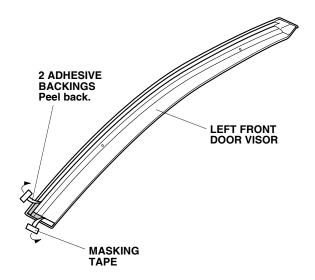
6. Place the door visor against the door, and adjust the visor so it lines up with the two front brackets.
