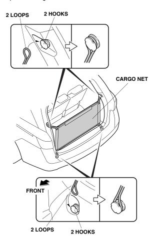
2. Secure four loops on the cargo net to the four hooks in the vehicle as shown.
