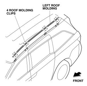
2. Open the tailgate halfway. Using a trim tool, pry up on the rear end of the left roof molding rear cover.
