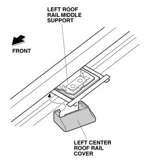
18. Install the left center roof rail cover to the left roof rail middle support as shown. Make sure that the left center roof rail cover has no clearance between the left roof rail middle support.
