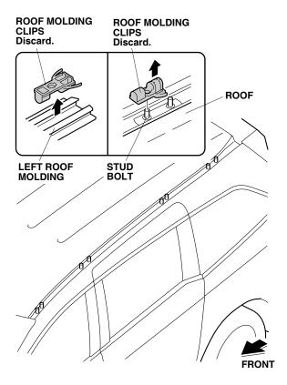
5. Remove any excess sealant from the stud bolts.
