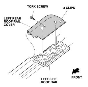
15. Secure the left rear roof rail cover to the left side roof rail with one Torx screw.
