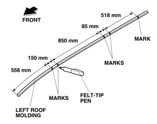
7. While wearing an eye protection, use an air saw to cut off the left roof molding at the marks made in step 6.
