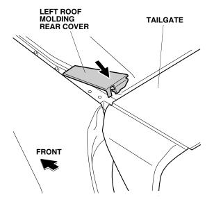
10. Reinstall the cut pieces of the left roof molding back onto the roof of the vehicle as shown.
