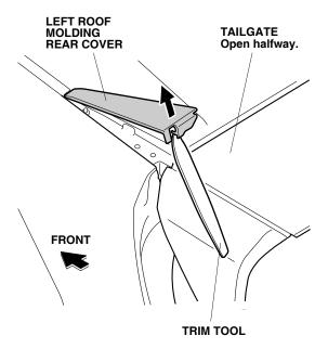
3. While wearing an eye protection, use an air saw to cut off the end of the left roof molding rear cover at the scribe line shown. Remove any burrs.
