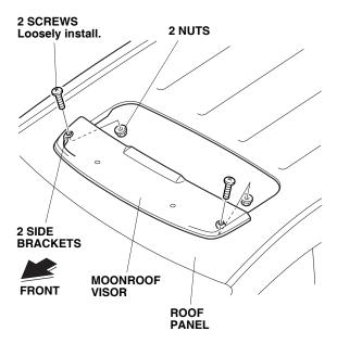
16. Adjust the moonroof visor so there is equal spacing on each side. Check that the rubber molding on the moonroof visor is not twisted or rolled under the visor and unfold if necessary.
