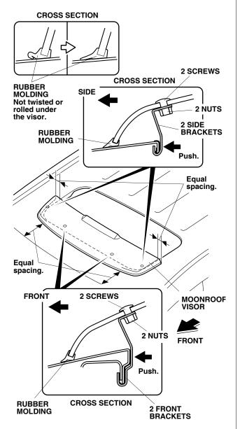
17. Tighten two screws and two nuts on each side of the vehicle first, then tighten two screws and two nuts on the front. Tighten while applying pressure so that there is no gap between the brackets and the roof panel. Torque the screws to 2 N·m (1.5 lbf·ft).
