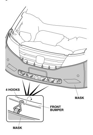
11. Secure the four hooks to the top of the lower grille in the areas shown.
