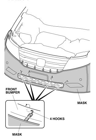
12. Secure the six hooks to the bottom of the front grille.
