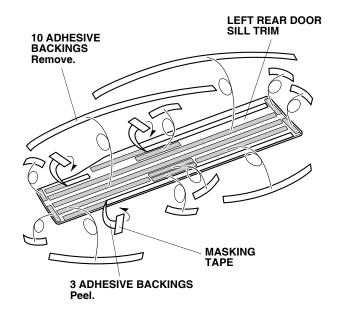
19. Remove the remaining adhesive backings.
