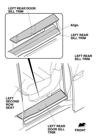
21. While applying light pressure against the left rear door sill trim, carefully remove the three adhesive backings.
