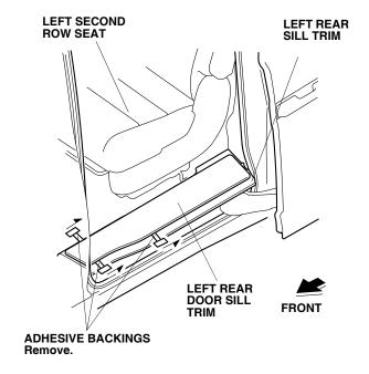
22. Using a rubber roller, apply pressure against the left rear door sill trim and roll from one end to the other.
