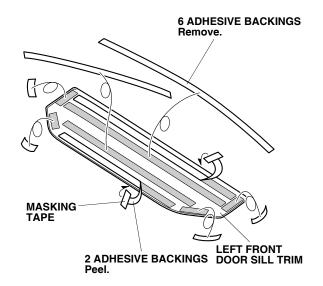
8. Remove the remaining adhesive backings.
