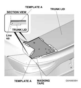
5. Using a felt-tip pen, mark the trunk lid through the five holes in template A.
