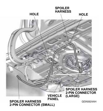
36. Unplug the vehicle 2-pin connector from the highmount brake light connector, and plug it into the spoiler harness 2-pin connector.
