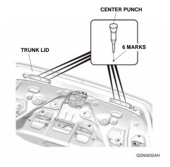
49. While wearing eye protection, drill the six center-punched marks on the trunk lid to 7.5 mm. First, drill with a 3 mm drill bit, then follow a 6 mm drill bit, and finish with a 7.5 mm drill bit.
