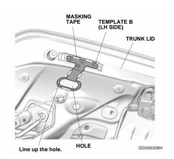
45. Using a felt-tip pen, mark the trunk lid through template B at the three holes on the template B.
