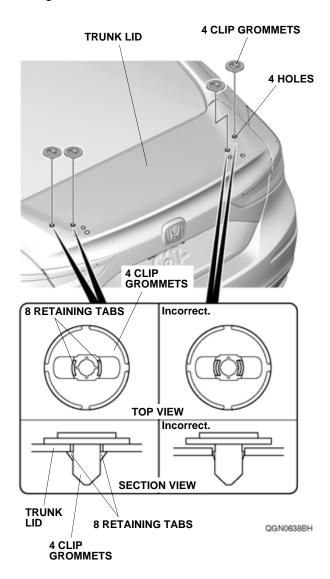
20. Install the four pins to the trunk spoiler.
