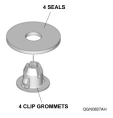
19. Install the four clip grommets to the four 8.5 mm holes on the trunk lid as shown.
