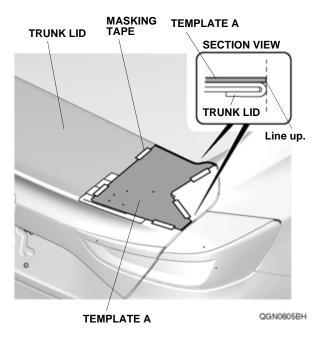
8. Using a felt-tip pen, mark the trunk lid through the four holes in template A.
