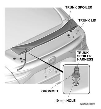
22. Remove two adhesive backings from the trunk spoiler.
