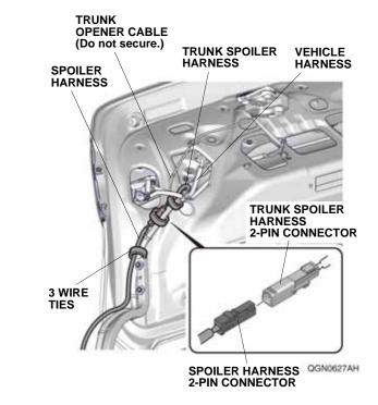
41. Secure the 2-pin connectors, trunk spoiler harness, and spoiler harness to the vehicle harness with three wire ties.
