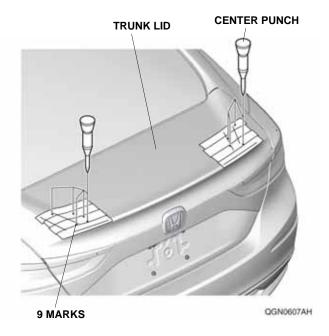
11. While wearing eye protection, drill the nine center-punched marks on the trunk lid with a 3 mm drill bit. NOTE: Wrap masking tape around the drill bit 10 mm (0.39 in.) from the tip, or use a drill stop. Make sure to drill the marks perpendicular to the trunk lid.
