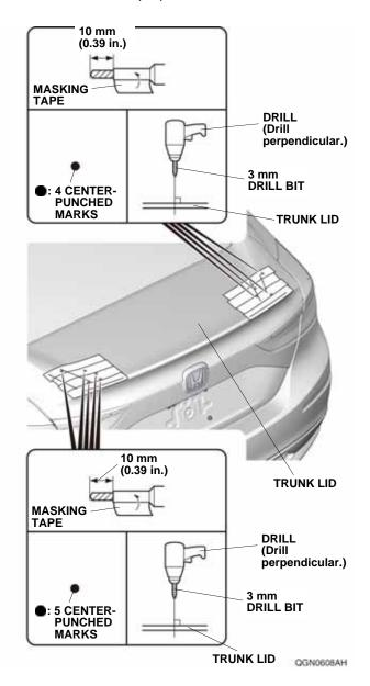
12. While wearing eye protection, use an 8.5 mm Rotabroach bit to drill the eight 3 mm holes as shown.
