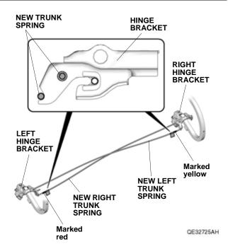
34. Install the center clip to the trunk springs.
