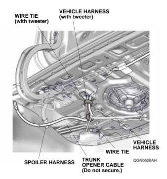
40. Plug the spoiler harness 2-pin connector into the trunk spoiler harness 2-pin connector.
