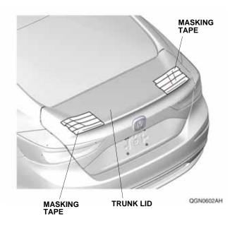
4. Place template A on the left side of the trunk lid, and line it up as shown. Then, secure it with masking tape.
