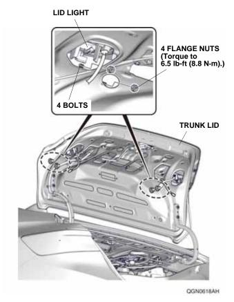
28. Plug the two vehicle 2-pin connectors into the left and right lid light. Secure the two vehicle harness clips to the trunk lid.
