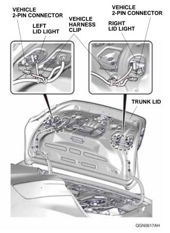
26. Release the two vehicle harness clips from the trunk lid as shown.
