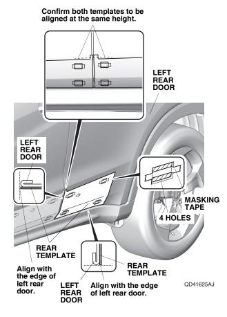
Using two alcohol swabs, clean the door surfaces above the templates where the body side moldings will attach. Allow the alcohol to dry before installing the body side moldings.
