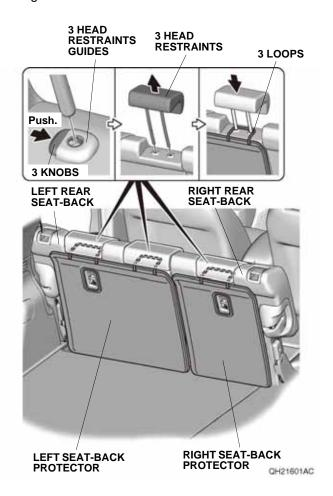
Fold down the left and right rear seat-backs, and peel back the cargo floor lid. Line up the left and right seat-back protectors with the tether anchor covers on the left and right rear seat-backs as shown.
