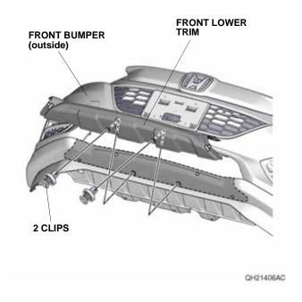
10. Secure the front lower trim to the front bumper with the four self-tapping screws.
