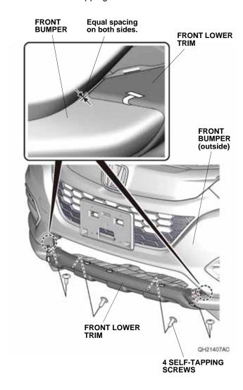
11. Install the front bumper lower grille to the front bumper. With the help of an assistant, install the front bumper.
