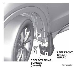
4. Remove the two self-tapping screws.
