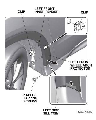
Remove two self-tapping screws and one clip. Pull out the left front wheel arch protector to release the clip.
