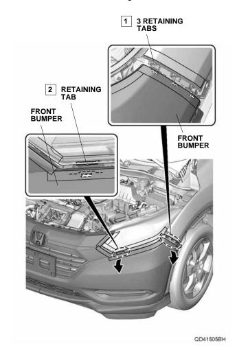
With the help of an assistant, remove the front bumper and unplug the vehicle connectors, if equipped. Place the front bumper on the blanket to prevent damage.
