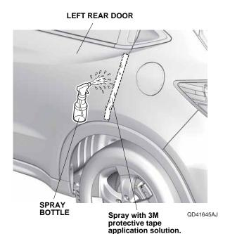
Open the left rear door. Peel back about 50 mm (1.97 in.) of adhesive backing from the left rear door edge film. Align the V-notch with the bottom of the character line on the left rear door as shown.
