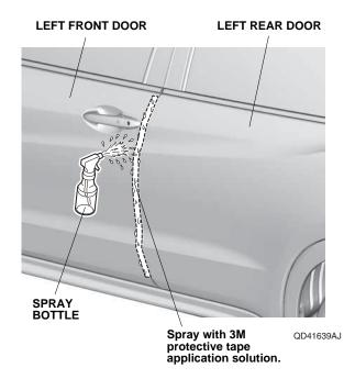
3. Open the left front door. Peel back about 50 mm (1.97 in.) of adhesive backing from the left front door edge film. Align the V-notch with the curved end on the left front door as shown.
