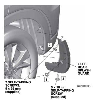
7. Turn the steering wheel fully clockwise, and repeat steps 2 through 6 to install the right splash guards.
