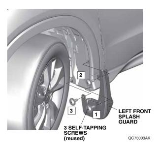
4. Remove the two self-tapping screws.
