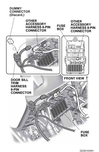
14. Plug the door sill trim harness 8-pin connector into the fuse box.
