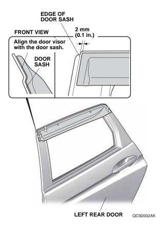
17. While applying light pressure against the left rear door visor, carefully remove the adhesive backings in the order shown. Use your finger to push up each bracket so there is no gap between the bracket and the door sash.
