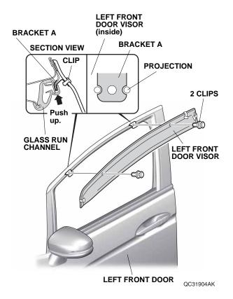
Adjust the left front door visor to the position as shown.
