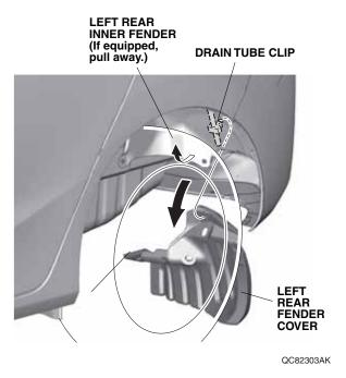
Locate the recessed mark. Using a pushpin, pierce the left rear fender cover at the recessed mark.
