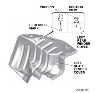
8. While wearing eye protection, drill the left rear fender cover at the pierced mark using a 3 mm drill bit first, then a 6 mm drill bit, 8 mm drill bit, and finish using a 10 mm drill bit.
