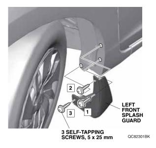
4. Turn the steering wheel clockwise, and repeat steps 2 and 3 to install the right front splash guard.
