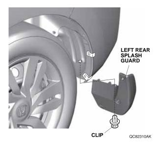
17. Secure the left rear splash guard the two 5 x 20 mm self-tapping screws in the order shown below.
