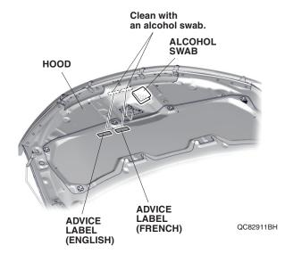
Remove the adhesive backings from two advice labels, and attach the advice labels to the hood as shown.
