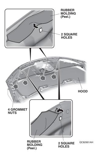
2. Using an alcohol swab, clean the four areas above the grommet nuts.
