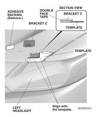
8. Turn the template over, and repeat steps 5 through 7 to install the bracket C on the right side of the vehicle.
