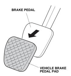
8. Separate the rubber pedal from the brake pedal cover. Install the new pedal pad on the brake pedal. Check that the pedal pad is installed on the brake pedal securely.
