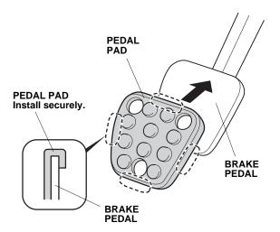
9. Align the pedal pad cover over the pedal pad.
