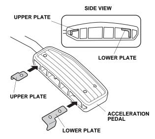
Place the accelerator pedal cover on the accelerator pedal. Insert one rivet through each hole in the pedal cover and into the plates. Using a rivet tool (MAR 3900), secure the accelerator plate to the accelerator pedal.
