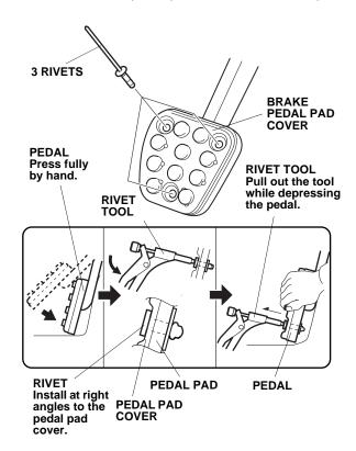
11. Repeat steps 7 thru 10 to install the pedal pad and pedal pad cover to the clutch pedal.
