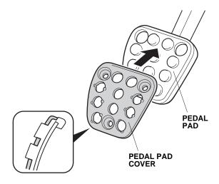
Insert one rivet through each hole in the pedal pad/ cover and into the brake pedal. Using the rivet tool, secure the brake pedal pad cover to the brake pedal.
