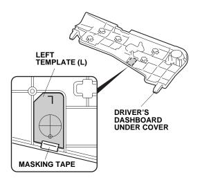
23. Using a pushpin, pierce the centers of the two scribe marks on the left template (L).
