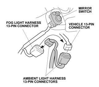
Using one wire tie, secure the excess ambient light harness and connector to the vehicle harness.
