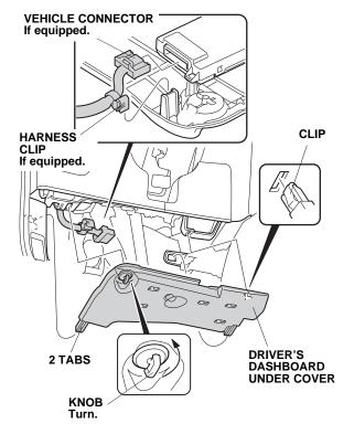
4. Remove the fuse access panel (two clips, five tabs, and two hooks). If equipped with fog lights, unplug the vehicle 5-pin connector and unclip the wire tie.
