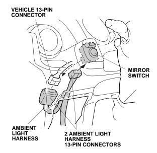
9. **With accessory fog lights:** Unplug the vehicle 13-pin connector from the fog light harness, and plug it to the ambient light harness 13-pin connector. Plug the other ambient light harness 13-pin connector into the fog light harness 13-pin connector.
