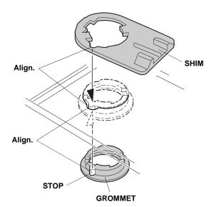
44. Attach the ambient light to the shim. Turn the ambient light clockwise to lock it in place.
