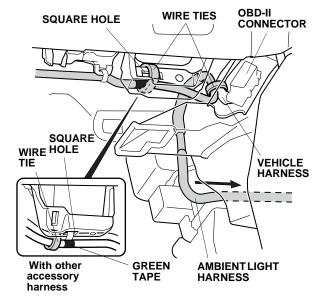
15. Using one wire tie, secure the ambient light harness to the OBD-II connector harness.
