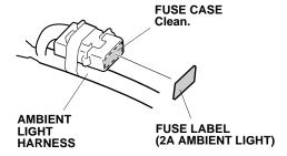
7. Attach the fuse label (2A AMBIENT LIGHT) to the fuse case on the ambient light harness.
