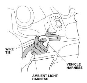
11. Using one wire tie, secure the ambient light harness to the square hole in the vehicle frame. (If another accessory harness is installed, secure the ambient light harness to the other accessory harness.)
