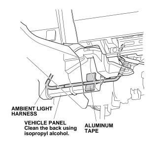
18. Use the aluminum tape to secure the ambient light harness to the back of the vehicle panel.
