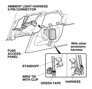
50. Using one wire tie with clip, secure the ambient light harness to the standoff on the fuse lid. (If another accessory harness is installed, secure the ambient light harness to the other accessory harness.).
