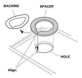
31. Align a grommet and shim through the hole as shown.
