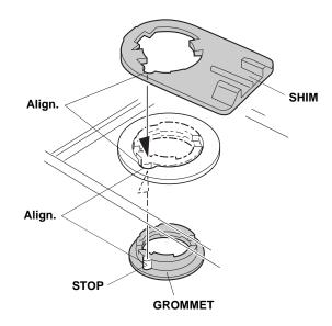
32. Attach the ambient light to the shim. Turn the ambient light clockwise to lock it in place.
