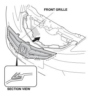
6. Install the four clips to the grille and the front bumper.
