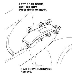
10. Repeat steps 6 thru 9 to install the right rear door switch panels.
