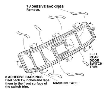
7. Using an alcohol swab, clean the surface where the left rear door switch trim will be installed.
