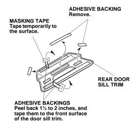
Using an alcohol swab, clean the surface where the rear door sill trim will be installed.
