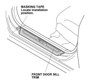
Peel back approximately 1½ to 2 inches of the adhesive backing from the two outer adhesive strips, and tape the ends to the front surface of the front door sill trim. Remove the remaining three pieces of adhesive backing from the trim.
