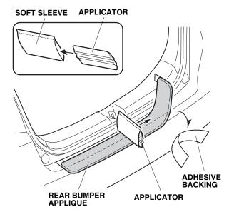
6. Remove the adhesive backing, and firmly press the rear bumper applique against the rear bumper.
